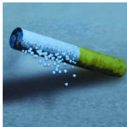
PIVOTING Gold-nickel nanorod tethered to silicon wafer precesses like a top in hydrogen peroxide solution when oxygen is generated at the nickel end.
