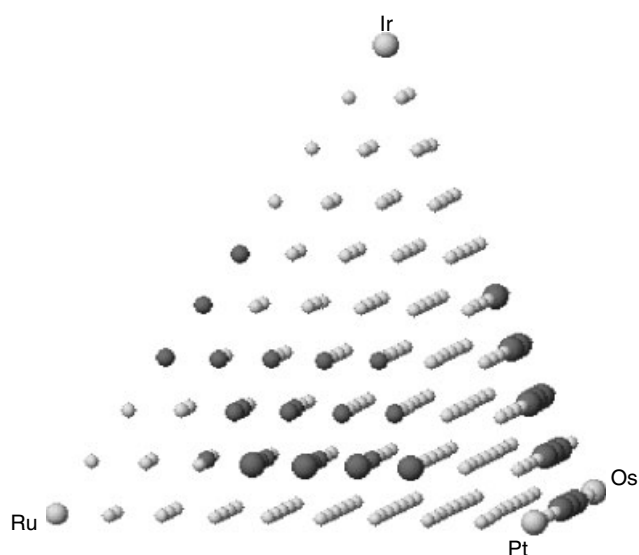
Figure 4. Re-folded activity map for oxygen evolution from a quaternary array of Pt/Ru/Os/Ir catalysts on Toray carbon paper. Large and small gray spheres indicate the onset of Ni-PTP fluorescence at +1350 and +1400 mV vs the normal hydrogen electrode (NHE), respectively.
