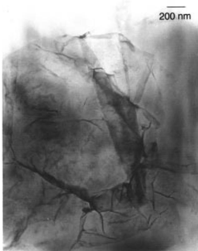
**Figure 1.** Transmission electron micrograph of colloidal graphite oxide particles.
